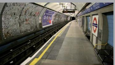
The Platform Humps at **Kings Cross Station** (to give level access to the Victoria Line trains) were installed at the end of May 2009. This is the latest phase of a project we have developed over the past five years, ensuring the platforms across the Victoria Line are DDA compliant.
