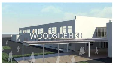
The main teaching block provides English, Maths, Languages and ICT Classrooms, together with Science Laboratories on the top floor and ICT Clusters in communal spaces. The building will be heated using a biomass wood pellet boiler and ventilated by a passive chimney system serving each classroom individually, to allow free air flow throughout the building.
